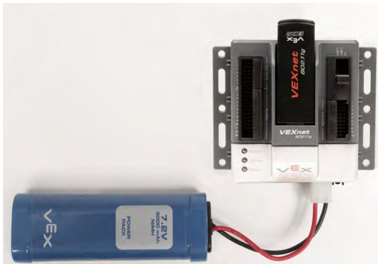
a. Attach a 7.2v battery and a VEXnet 802.11g key to the VEX Cortex as shown.
