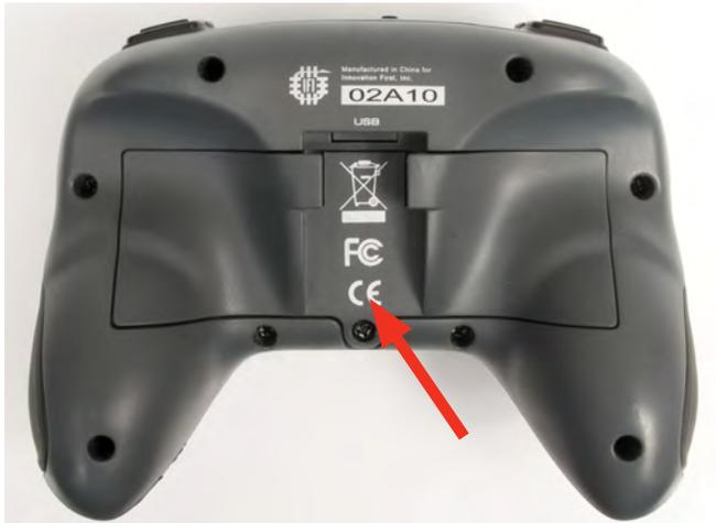
b. Install six identical batteries as shown. Use Alkaline, Ni-Cad or Ni-MH chemistries, but DO NOT mix different chemistry batteries. Charge rechargeable batteries only with a quality charger designed for your battery chemistry.
