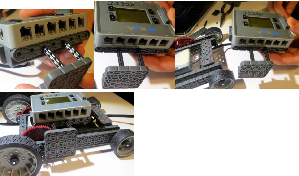
Step 4 Attach wires to brain. Note ports: one side is port 7 the other side is 6.
