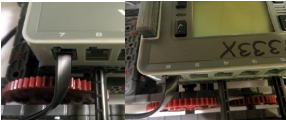
Step 4 Attach wires to brain. Note ports: one side is port 7 the other side is 6.
