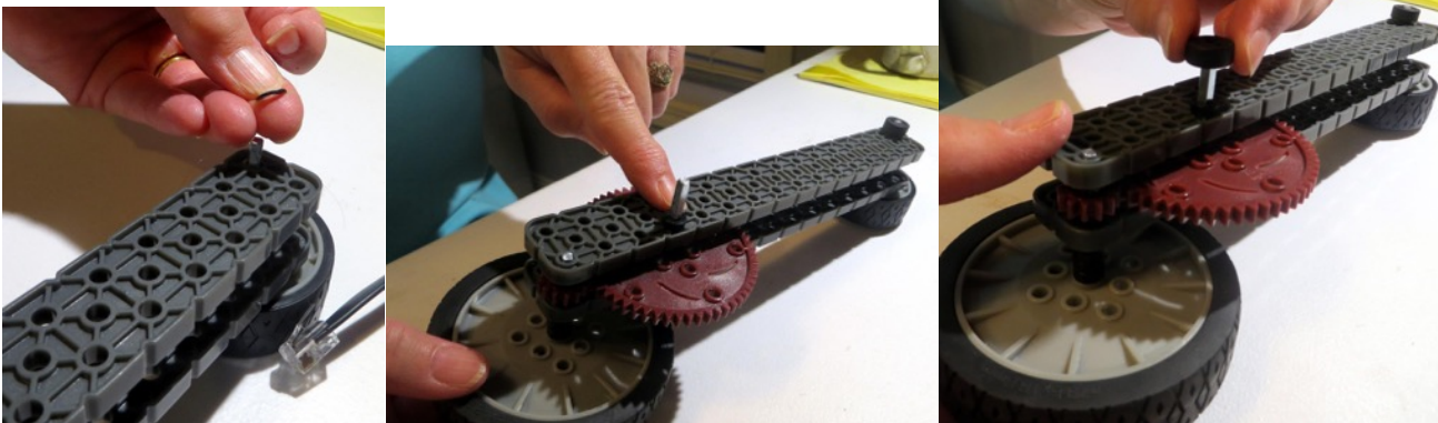
Step 5. Motor mount. (3) 2x standoffs, (1) motor, (1) smart cable
