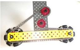
4 Bring the one end of the chain to where the other end left off. The chain should be a little long. (If not add links to make it too long). Pull the chain to make it taut, and note which link should be removed to make it the right size.
