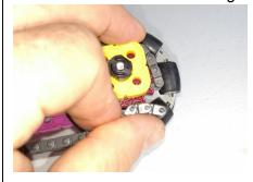
3 Run the chain between the sprockets to make an S shape
