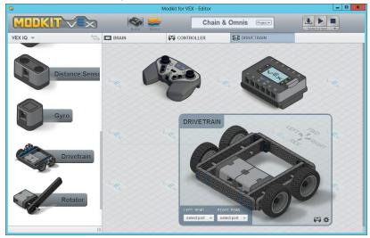
2. Configure the ports for the drivetrain. Which ports do the wires from the motors go into the brain? You can use any ports you want. But if you use ports 6 & 7 then the Driver Control program will work too.
