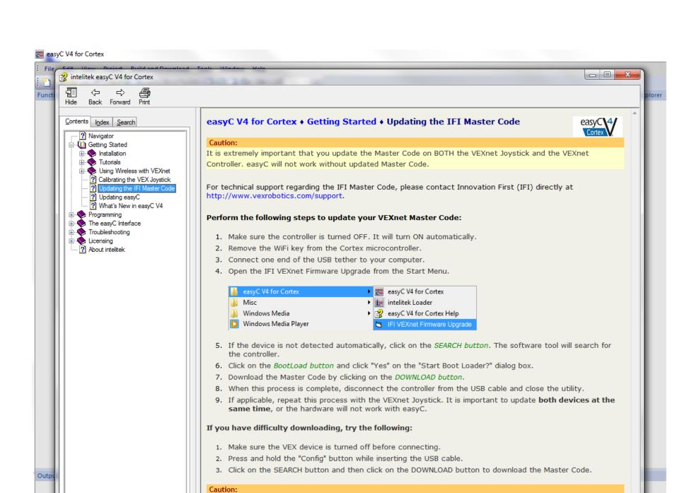
If it is necessary to use the Bootload option, the joystick will need to be re-calibrated when you are done. If none of these solutions work, contact Innovation First at http://www.vexrobotics.com/support.
