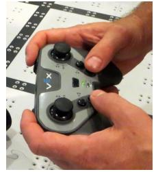
Simultaneously press the lower E & F buttons and the upper R & L buttons to move backwards
