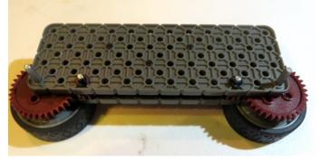
Step 5. Motor mount. (12) normal connectors, (2) thin washers, (2) motors
