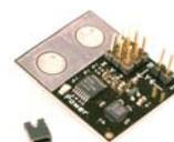
accelerometer, senses X, Y and Z acceleration
