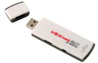
VEXnet key, NOT a usb drive, but a 2.4GHz transmitter/receiver
