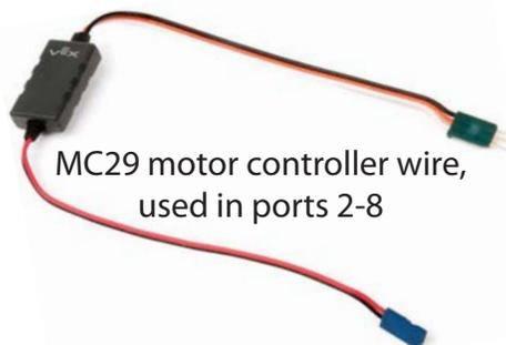
MC29 motor controller wire, used in ports 2-8
