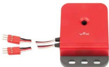
optical shaft encoder, counts shaft rotations
