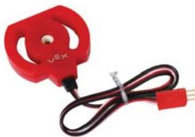
potentiometer, senses shaft angle
