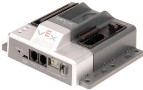
Cortex microcontroller, ARM cpu with multiple I/O ports, stores and runs programs
