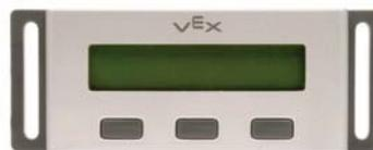
LCD display, connects to UART port with a special cable
