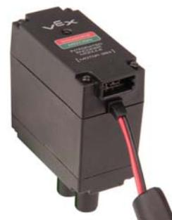
393 motor with encoder back, counts motor rotations, allows PID control
