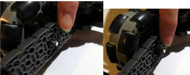
Step 5. Attach motors. (4) motors, (16) normal connectors, (4) thin washers, (4) medium length smart cables
