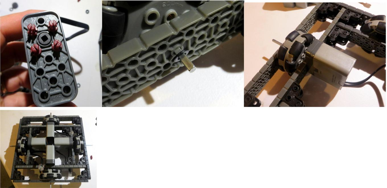
Step 6. Attach brain, (4) 4x standoffs, (2) 1x10 beam, (4) 2x2 brackets, (8) normal connectors
