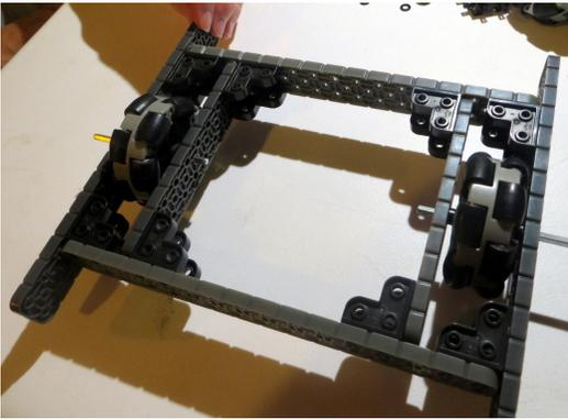
Step 4. Add second set of wheels. (8) corner brackets, (2) omni wheels, (2) #3 shafts, (6) rubber washers, (2) spacer washers, (2) thin washers, (2) 2x16 beams
