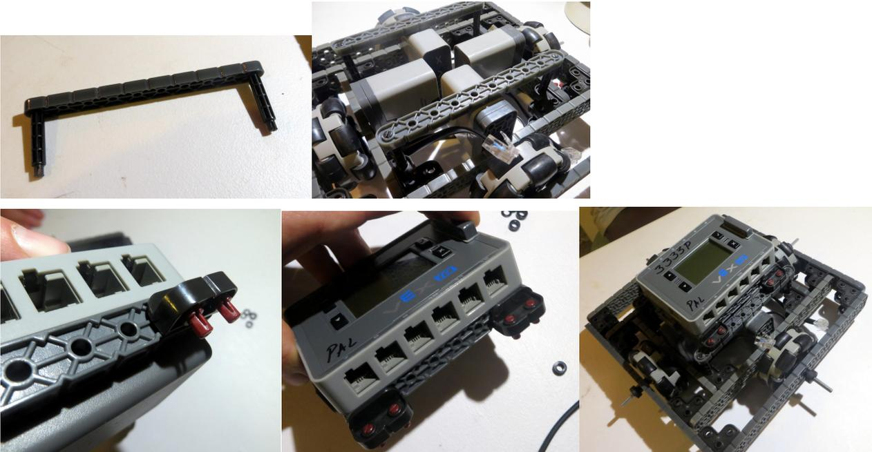
Step 8. Attach the smart cables to the brain.
