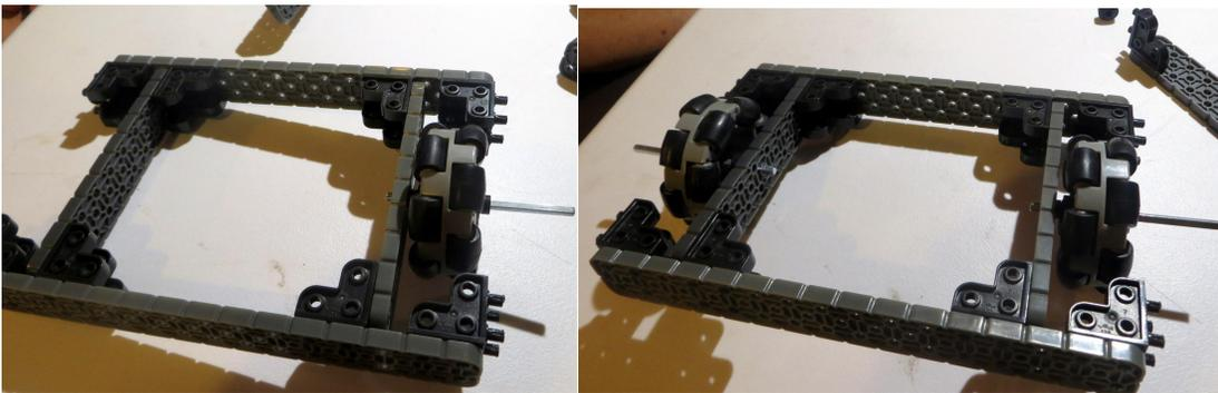
Step 3. Add supports and lock in wheels. (2) 2x16 beams, (2) thin washers, (2) rubber washers
