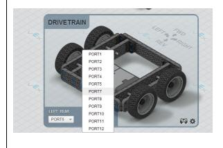
3. If you want the back of the robot to be where the brain is then reverse the direction of the motors. Click on the gear icon (configure) and then click the "rev" checkbox on each motor.
