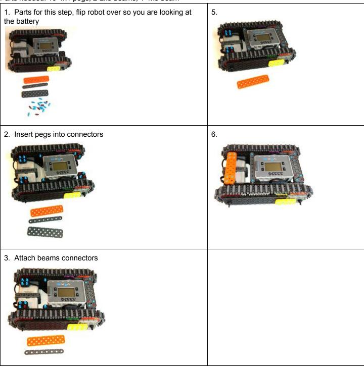
Parts needed: 10-1x1 pegs, 3-2x8 beams
