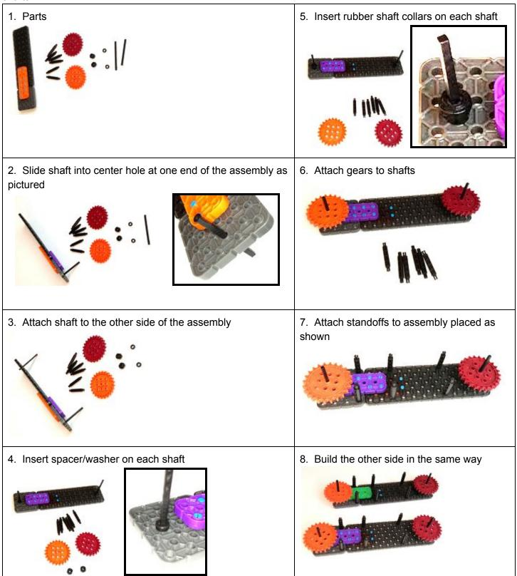
Parts needed: 4-rubber collars, 2-washer spacers, 8-1x2 pegs, 2-2x4 beams, 1-4x4 plate, 1-4x12 plate
