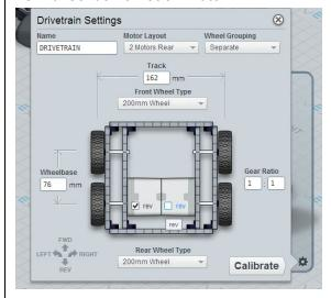
4. For the Wheel Grouping section select "Connected". You can optionally measure and input the wheelbase, but the program will work without that
