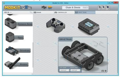
2. Configure the ports for the drivetrain. Which ports do the wires from the motors go into the brain?
