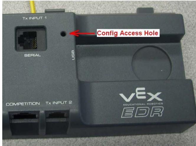
2. VEXnet Receiver CONFIG Switch Access Hole
