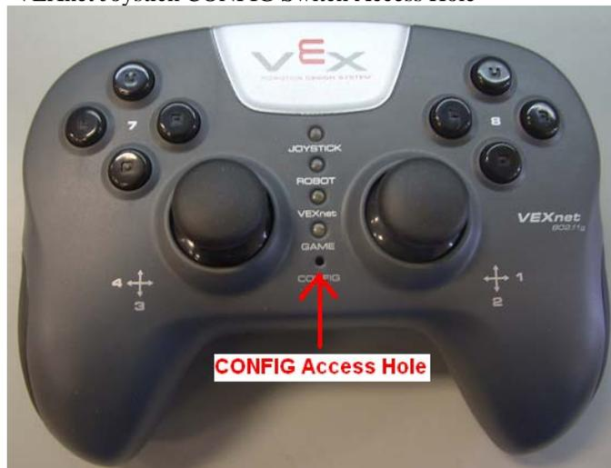
2. VEXnet CORTEX CONFIG Switch Access Hole
