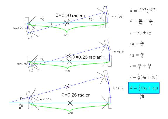
Our robot has an encoder on each wheel, so we combine formula (1) for wheels  $S_0$  and  $S_2$ , with the same formula for wheels  $S_1$  and  $S_3$  giving us formula (2) below. The effect of this is an average of the measurement of the two wheel pairs. Finally, since the robot is not a true square and there may be imperfection in the placement of the wheels, it is most practical to determine a calibration constant "K" experimentally. Formula (2) below tracks the angle of the robot.
