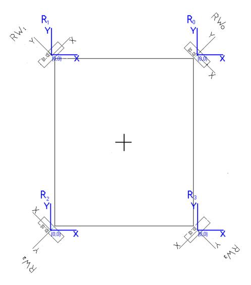
We use vectors to track the relative motion of the wheels. The vectors used are column vectors. The top element is the X value or the vector and the bottom element is the Y value. Column vectors are preferred because they are compatible with <u>matrix</u> <u>multiplication</u> [ref 11]. The Delta " $\Delta$ " in the formulas below represents "change in", and is used to indicate relative motion of the wheel during the 25 millisecond (mS) program loop. A millisecond is 1/1000 of a second.
