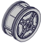
2x Wide, Ø48.5mm Diameter Hub
