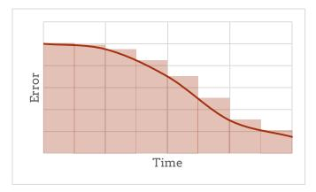
The "area under the curve" for each cycle of our loop is going to be the current error, multiplied by the time it takes for that cycle of the loop. It's a rough approximation, but it works fine for us with such slim slices of time.
